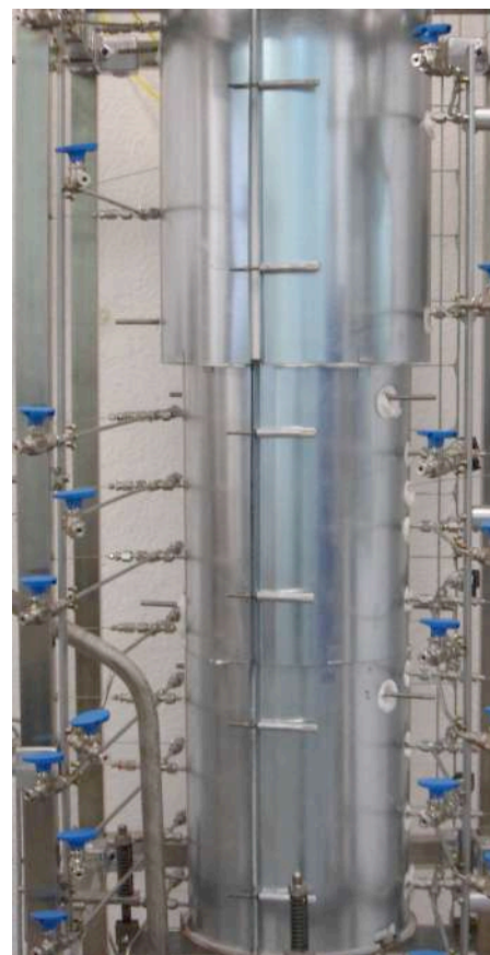
Fluidized Bed pilot plant (3kg/h of biomass)
