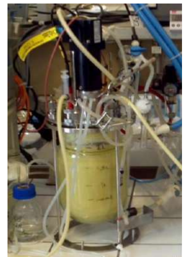
Batch fermentation process of micro-organisms carried out in a fully instrumented bioreactor
