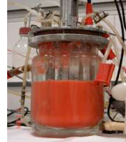
Sporobolomyces ruberrimus growth kinetics and carotenoid production on 3 L bioreactor
