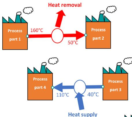
To illustrate the concept, let us consider a schematic process involving two heat exchangers: a hot stream is cooled from 160 to 50 °C while a cold stream is heated from 40 °C to 110 °C.
