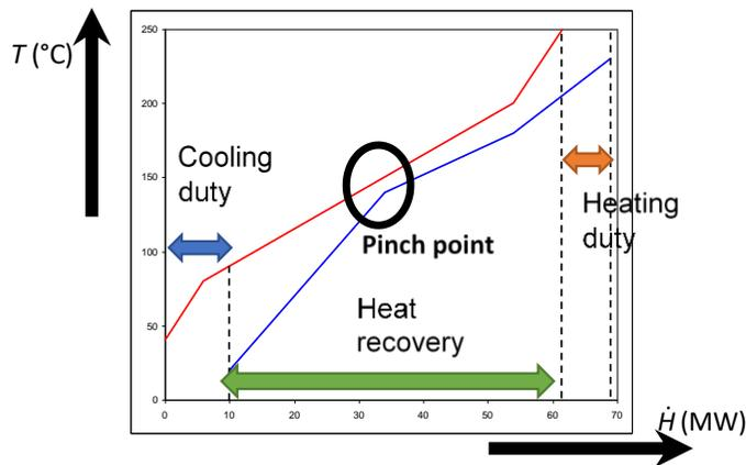
The user specifies the value of the pinch which is the lower difference between the hot and cold composite curves. These are then shifted horizontally until the specified pinch is reached. **The overlap between the composite curves represents the maximal amount of heat recovery possible within the process.** The corresponding net of heat exchangers can be then deduced by applying complex algorithms.
