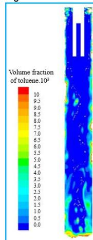
Hydrodynamic study: cyclonic separator (for the recovery of the organic solvent (toluene) from the CO<sub>2</sub> + organic solvent mixture issued from the aerogel drying process).
