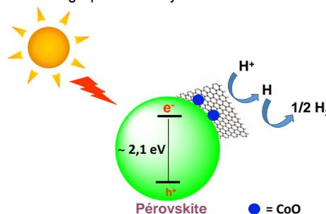
Figure 2: Schematic representation of the prototype device.
